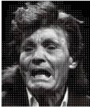
Figure 2: Image with overlay of its HOG representation.
